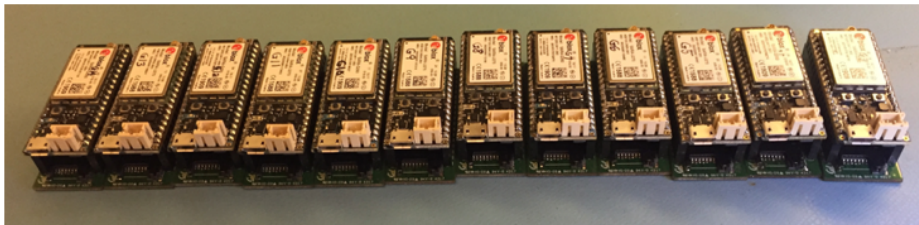
12 Plug-load sensors used in small scale deployment
