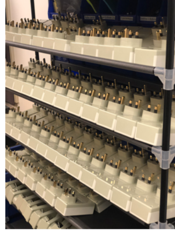
A shelf of assembled plug-load sensors
